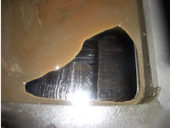
Photo 3: Lead-free solder pot with wave not running showing MS2 on the shiny dross free solder surface.
