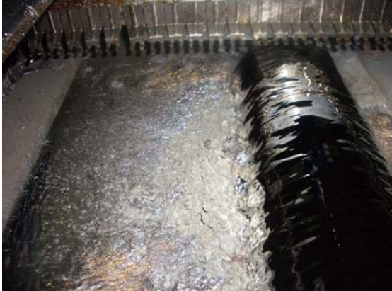
Photo 1: Lead-free solder pot with normal build-up of dross.
