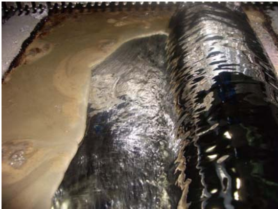
Photo 2: Lead-free solder pot with MS2 and no dross.
